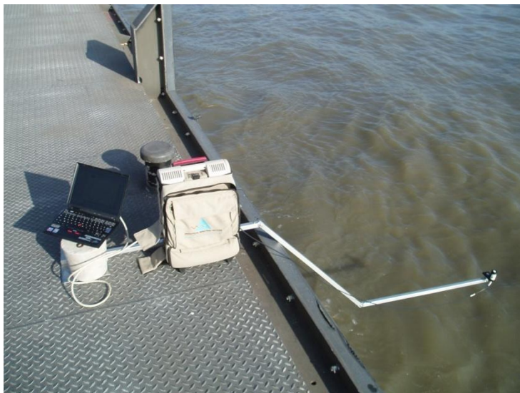
Figure 8 - ASD equipment measuring the Sky radiance
