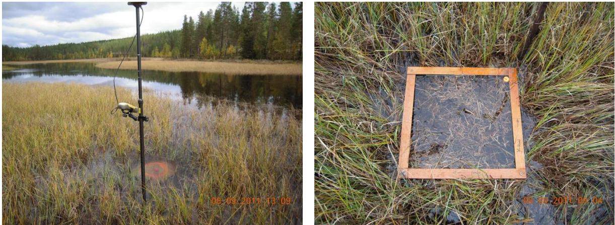
Figure 3-2-2. Measurement of control points and example of biomass sampling.
