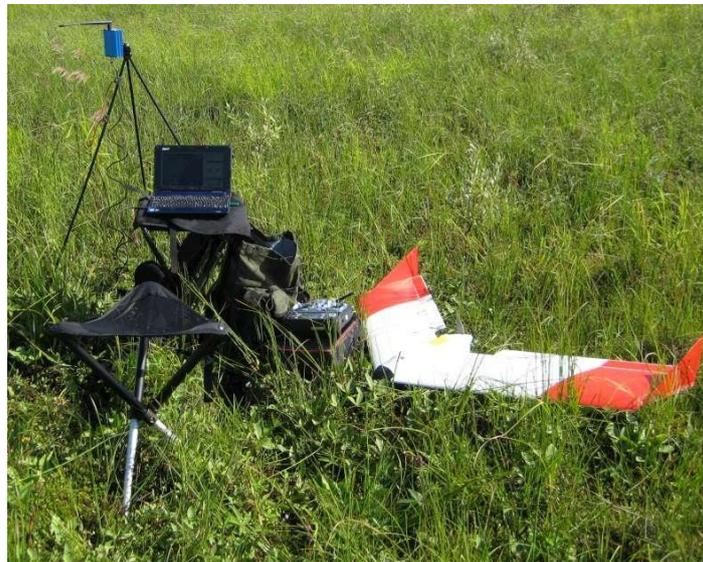
**Figure 3-2-1. Unmanned aircraft system (UAS) consisting of a remotely controlled airplane (wingspan 1.2 m) with a digital camera and a ground control station with mission planning and flight control software.**
