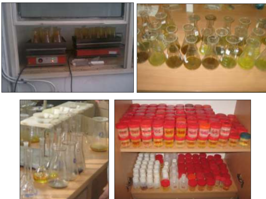
Figure 4-6. Soil/sediment sample digestion.
