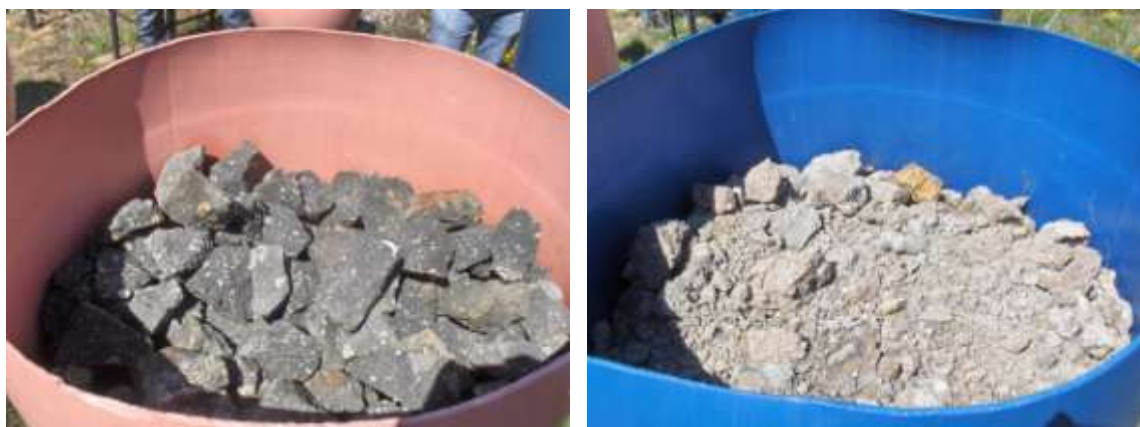
Figure 3-25. Plastic barrels with rock samples used for the kinetic test.
