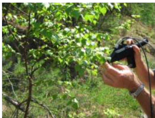
Figure 6-33. Leaf spectral sampling with the plant-probe.
