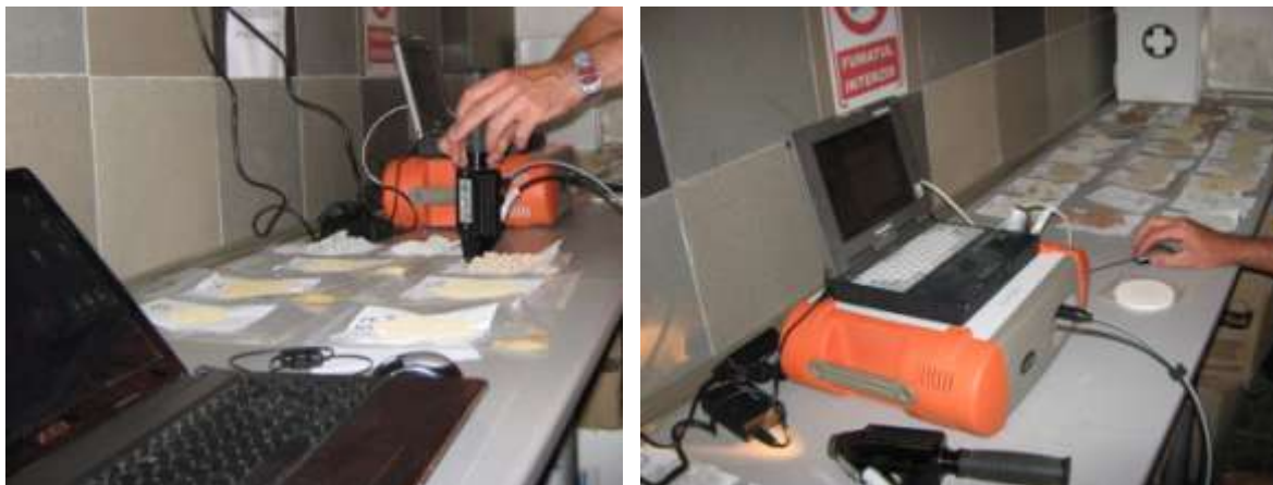
Figure 5-8. Hyperspectral measurements of soil samples by the ASD spectrometer in the lab.
