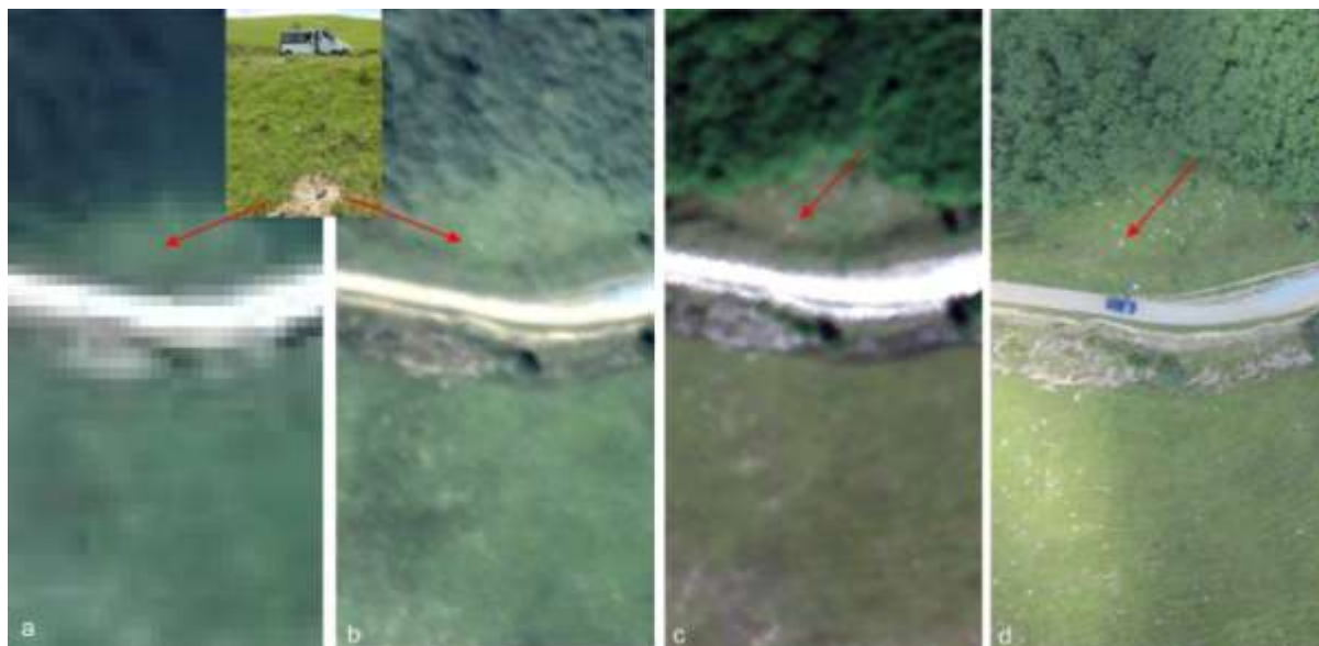
Figure 5-12. Comparison of Worldview2 Multispectral (2m resolution), WV2-pansharpened multispectral (50 cm resolution), Hyperspectral VNIR (50 cm resolution) and Smartplanes image (4 cm resolution). The red arrows point to the location of the soil exposure shown in the photograph. This type of soil exposure is found frequently in grass lands used for grazing.
