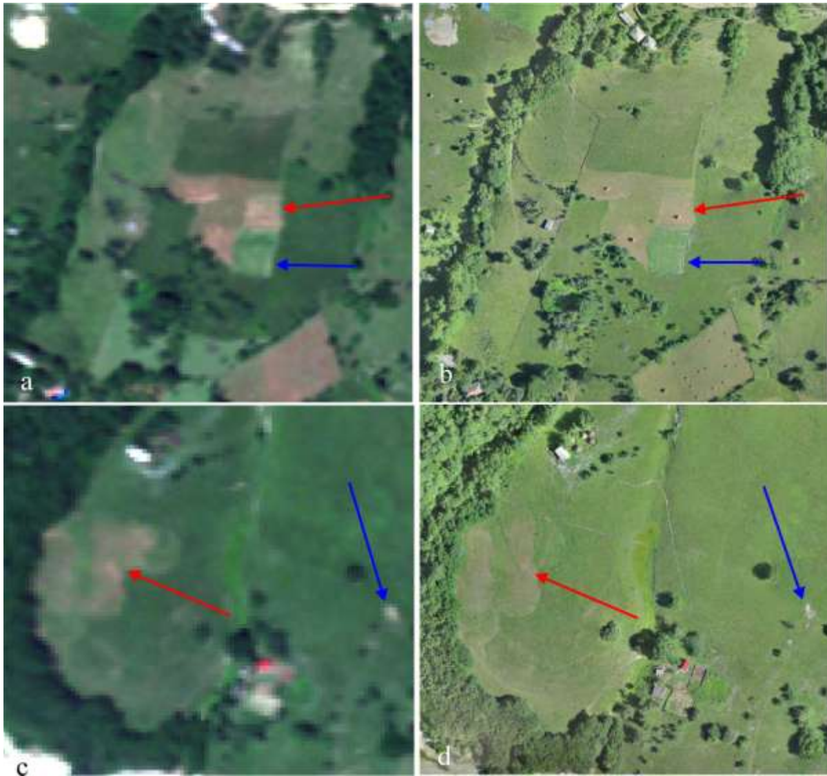
Figure 6-14. Comparison of the July 2012 WV2 imagery and the Smartplanes imagery for various types of soil exposures a-b: red arrows mark examples of recently cut, and dried grasslands. Hay stacks are clearly visible on the Smartplanes image; Blue arrows indicate exposed soil in a crop field. c-d: Red arrows mark examples areas that appear to be in the process of being cut. Blue arrows mark examples of exposed soil.
