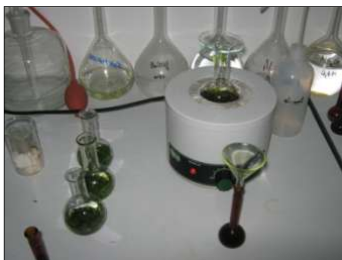
Figure 4-14. The process of heating and separation using FALC Heating Mantles.
