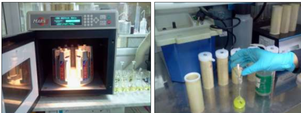
Figure 4-10. Samples digestion (left: during digestion; right: after digestion).
