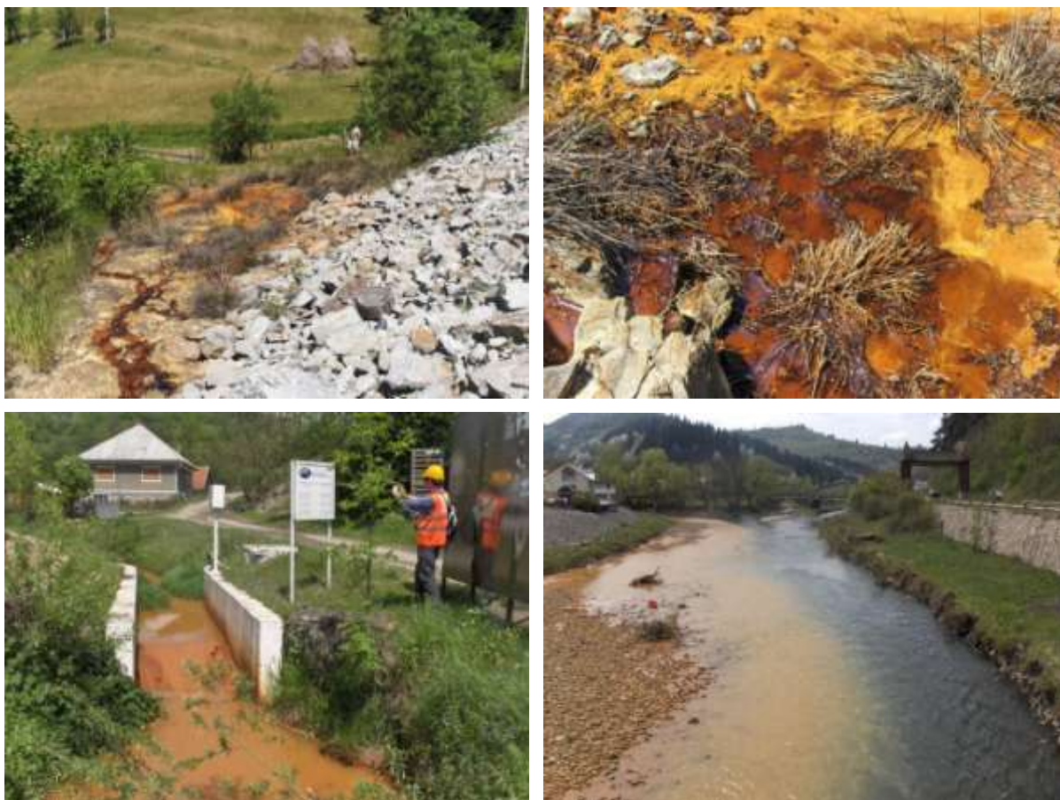
Figure 3-12. (a) Acid mine drainage downstream of Saliste tailings dam; (b) Fe-hydroxides and gypsum in the seepage area, Saliste tailings dam; (c) Weir on Saliste Valley, close to the confluence with Abrud River. (d) Mixing between the AMD-polluted waters of Abrud River (left) and the relatively clean waters of Aries River (downstream Campeni).
