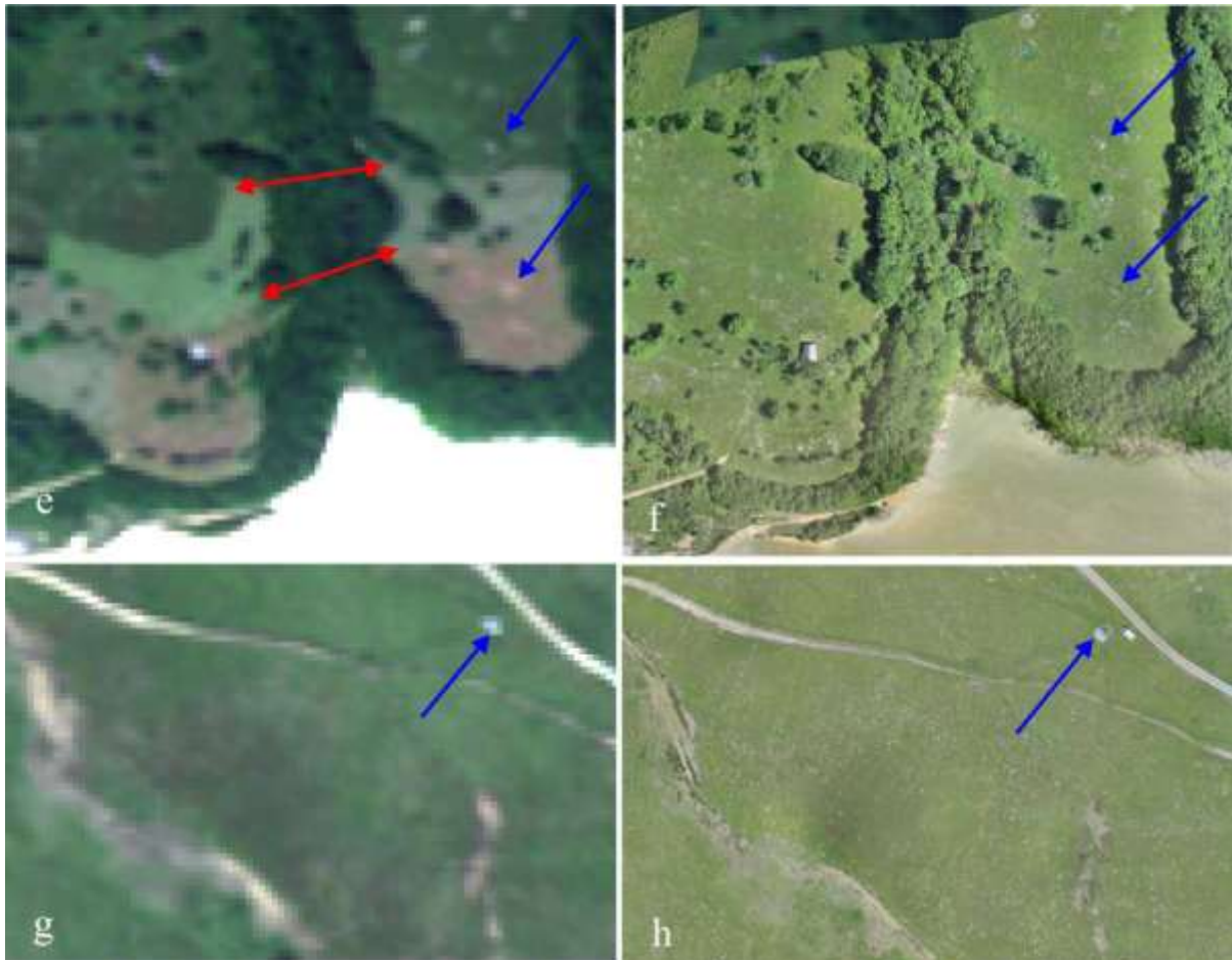
Figure 6-15 e-f: The red arrows mark a strange zoning in the grasslands for the WV2-image. This zoning is not visible in the Smartplanes image. We suspect that in this area the cutting of the grass is still in progress, and that in the brown areas grass has been cut in the four days lapse between the acquisitions of the two datasets, whereas the greener part has probably been cut more recently. The blue arrows mark exposure of rocks and soil. g-h: image of typical grazing land with very short grass, and many small spots with exposed soil (see also figure 6-12). The blue arrow marks a small pile of gravel. The other white spot on the Smartplanes image is our field-van.
