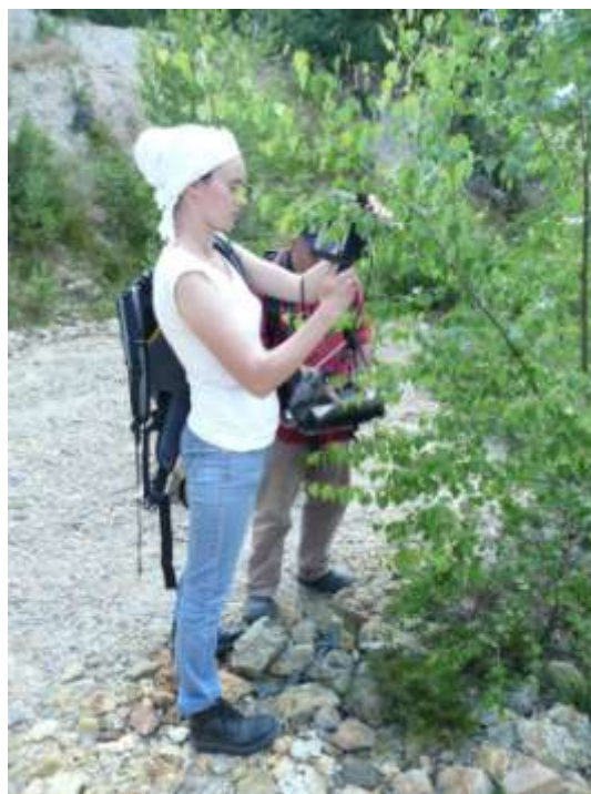
Figure 5-9. Hyperspectral measurements on leaves in the field
