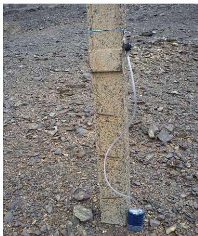
Fig. 4.3 Air sampling apparatus set up downwind from the Karabash smelter
