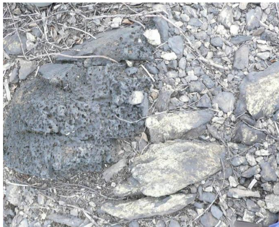
Fig. 5.23 Photo taken about 5 km southwest of the Karabash smelter. Clearly visible are the holes where mafic minerals such as olivine and pyroxenes have been leached out. The composition of the black varnish has not been analysed.
