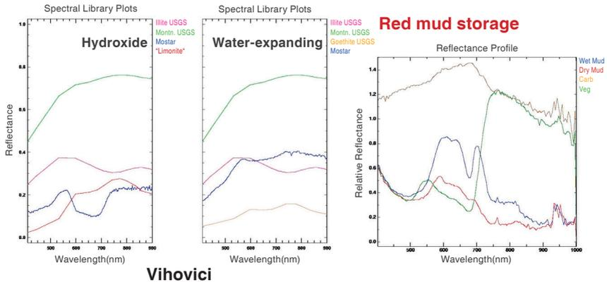
Figure 7 – Some reflectance spectra derived from the airborne hyperspectral data and compared with various spectral library mineral samples to aid in mapping and classification
