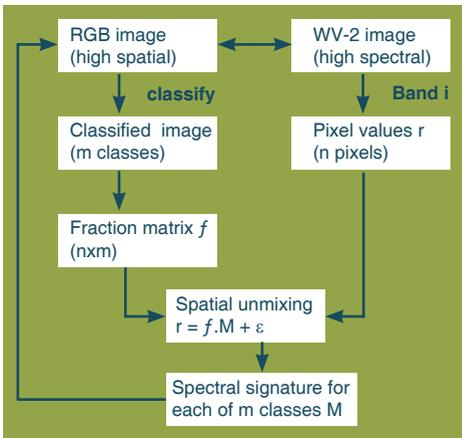
Figure 8 – Schematic overview of the spatial unmixing technique
