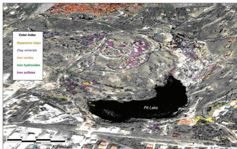
Figure 6 – View of bauxite-ore waste containment facility imaged with hyperspectral data and analyzed with red-mud index derived from the Hungarian spill.
